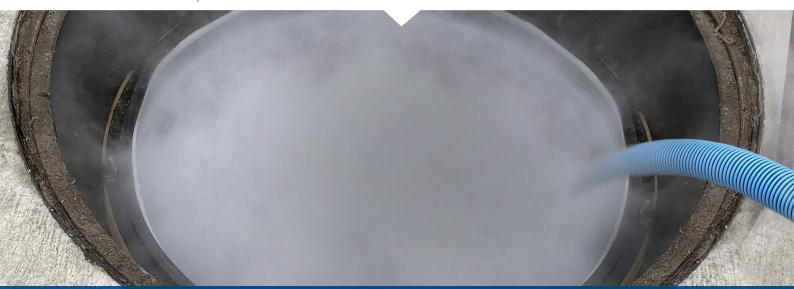
Dri-sump® uses lasers and aerosol fog to find leaks in all types of sumps and spill buckets. It's an EPA-approved containment-tightness testing technology that delivers digitally recorded pinpoint testing accuracy to 0.05 gph in just 60 seconds.
